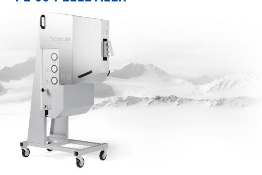
DRY ICE OUTPUT Up to 176 lb/h (80 kg/h) of dry ice pellets
